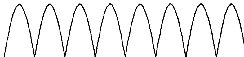
(c) Full-wave rectification
