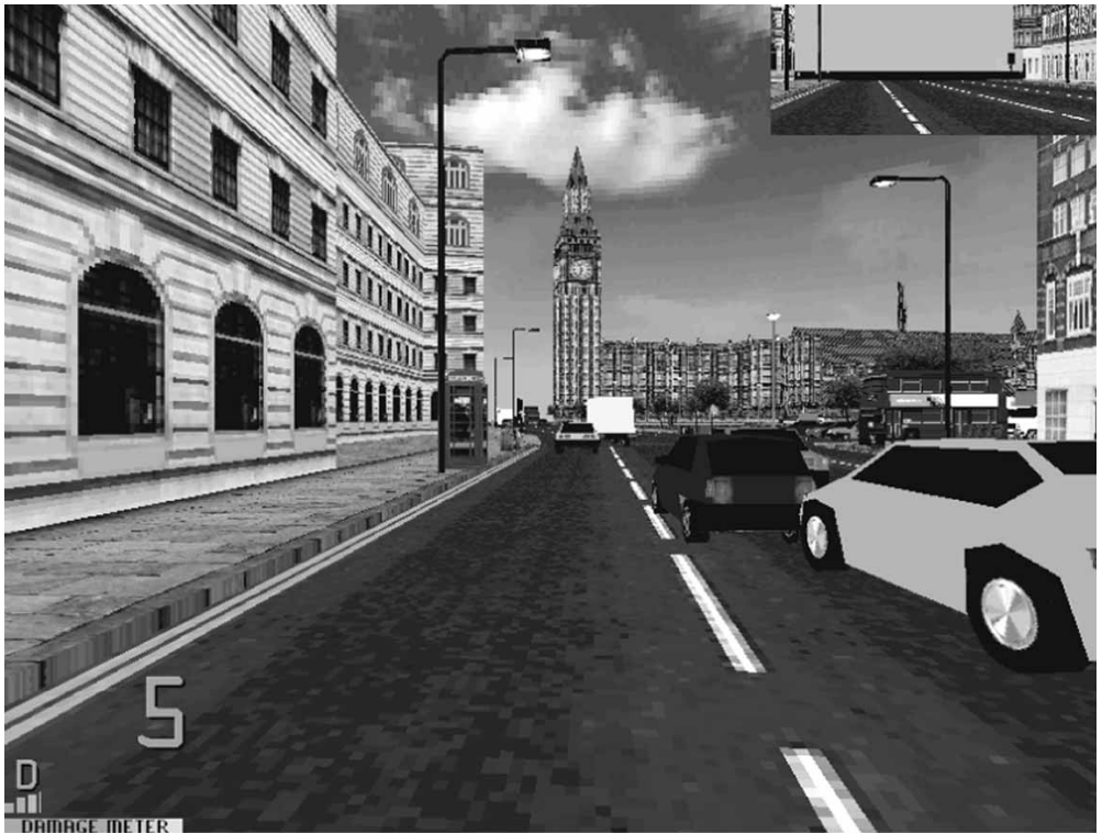
Figure 1. A sample screen taken from a simulated drive. The rear-view mirror is represented at the top right of the screen. The number in the bottom left corner is a measure of speed (screen shot reprinted by permission from Microsoft Corporation).
